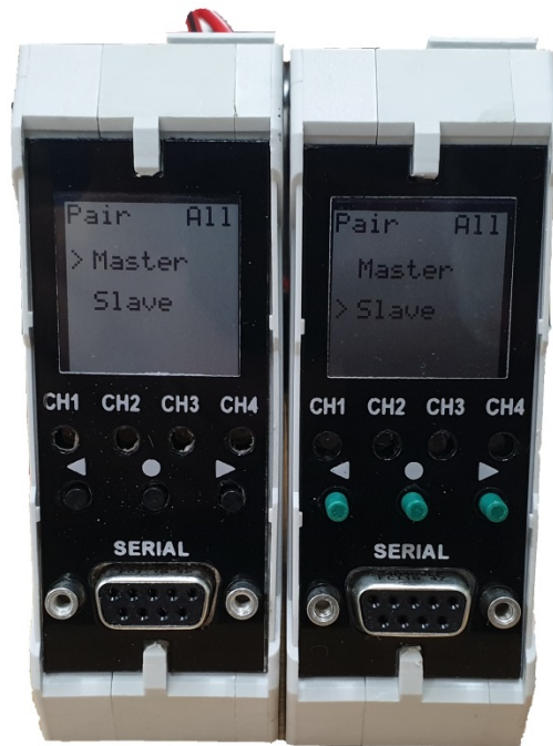
Fig 21: Two XL-CCCs configured for synchronised scanning.
