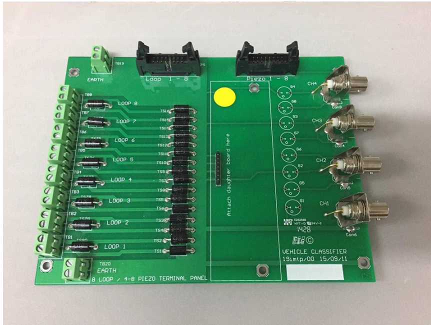
Figure 1.2: Excel Technology Loop Termination Panel.
