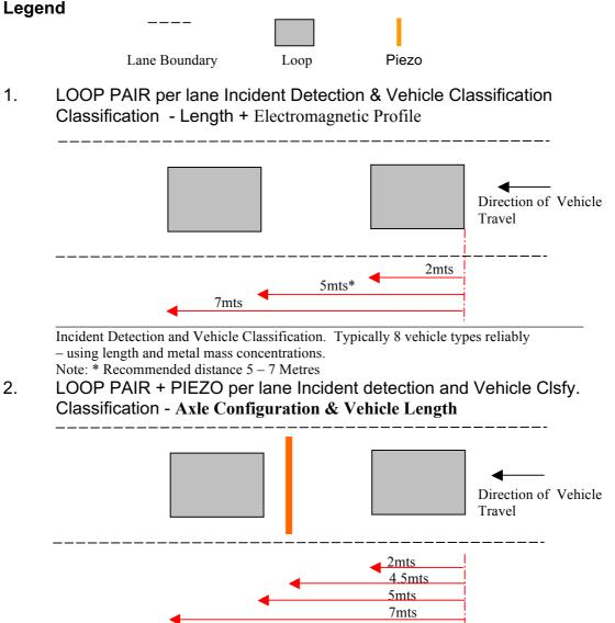
Incident Detection, Vehicle Classification Typically 14 to 21+ vehicle types and vehicle loaded unloaded status (binary weight)
