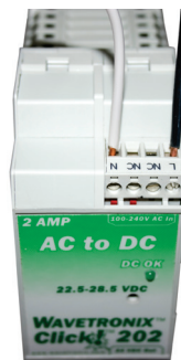
Figure 2.6 – Wiring AC Power into the Click 201/202
