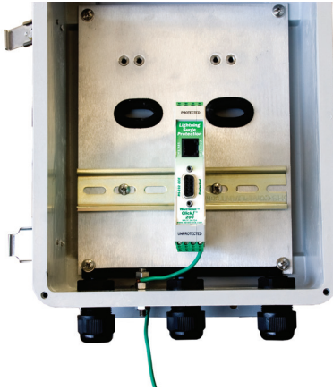
Figure 2.4 - Earth Ground Connections
