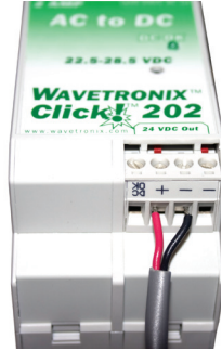
Figure 2.7 – Wiring DC Power Out of the Click 201/202
