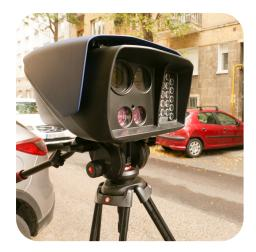
Adaptive Recognition S1 is a mobile no-staff speed and traffic enforcement device with onboard ANPR. It is capable of detecting traffic violations like the abuse of bus lanes and measuring speed from a whopping distance of 1,200 meters (4,000 feet).
